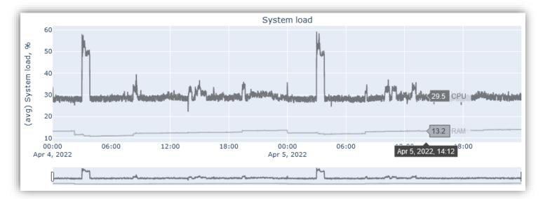
• System load chart shows system CPU load (in %) and RAM memory usage (in %)
